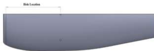
Figure 2.1 Engine nacelle micro porous Hole-location.
