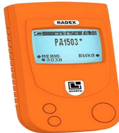
Figure 2 shows the RADEX 1503+ Geiger-Müller counter used in this fieldwork.
