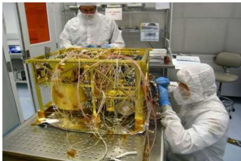
The gold-plated Sample Analysis on Mars contains three instruments that make the measurements of organics and methane. IMAGE CREDIT: NASA/GODDARD SPACE FLIGHT CENTER.
