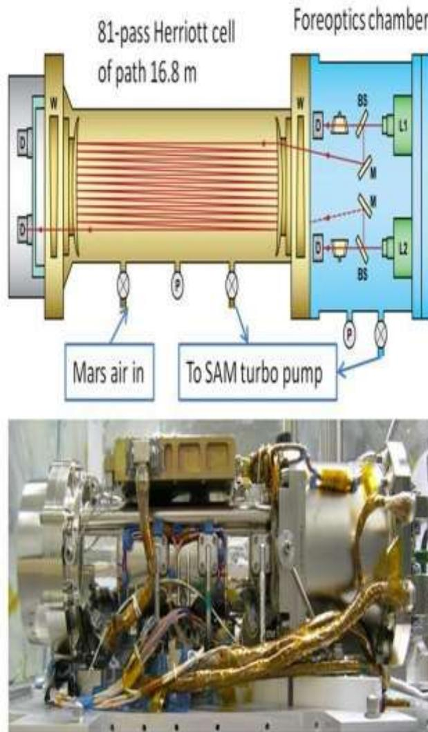
By measuring absorption of light at specific wavelengths, the tunable laser spectrometer on Curiosity measures concentrations of methane, carbon dioxide and water vapor in the Martian atmosphere. IMAGE CREDIT: NASA.
