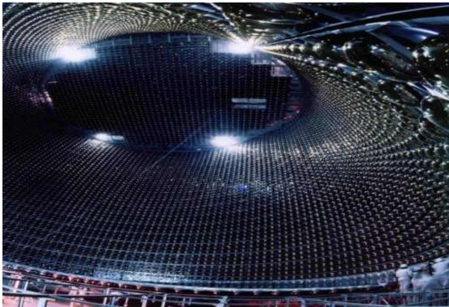
Figure1(a) shows Super-Kamiokande Detector courtesykamiokaObservatory,ICRR(Institute for Cosmic Rays Research), The University of Tokyo. Is kind of Neutrino detector Super Kamiokande which detect muons in the Water.
