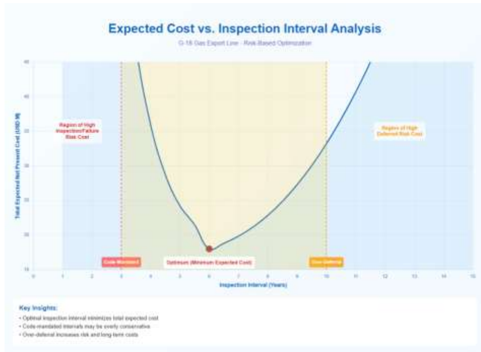
Figure. Expected cost optimization curve for inspection planning, illustrating the cost penalty of both overly conservative (code) and overly deferred intervals.
