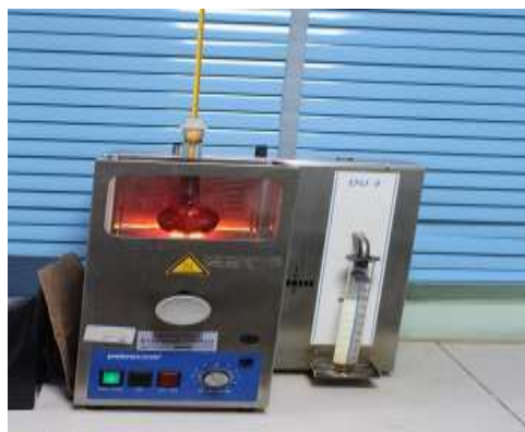
Figure 8: Petrotest DU 4 Distillation Unit
