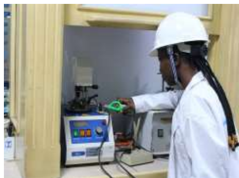
Figure 6: Abel Closed Cup Flash Point Machine
