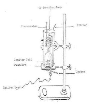
Fig. 1: Fuel/Food Calorimeter: Apparatus for measuring calorific Value
