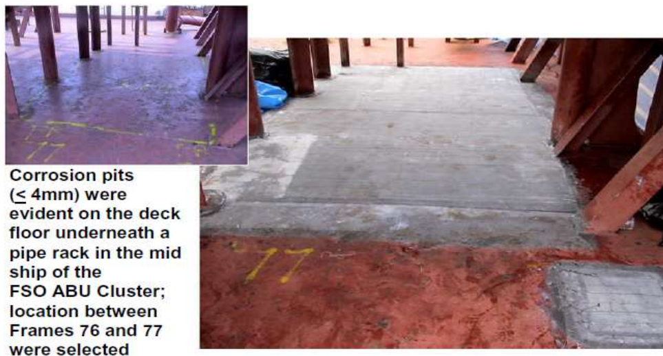
Figure (7): Repair of the corroded deck plate of the FSO Abu Cluster [70].
