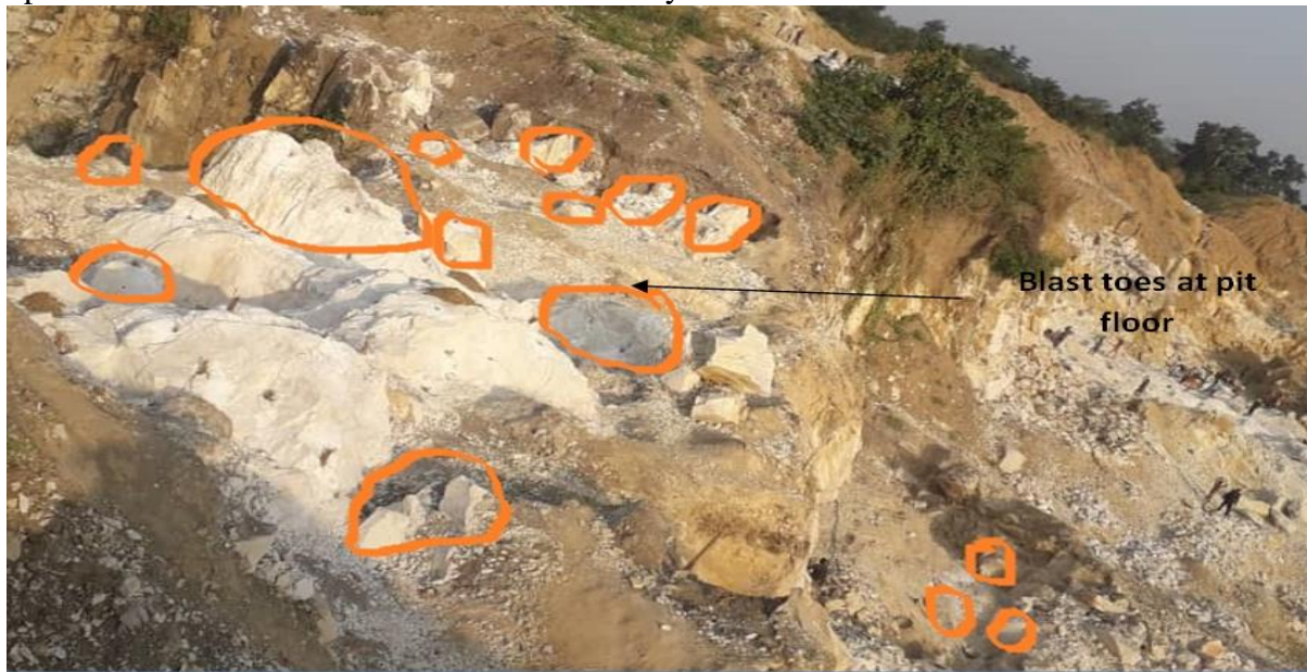
Fig. 1 Evidence of toes after loading operation at the case stud quarry pit
