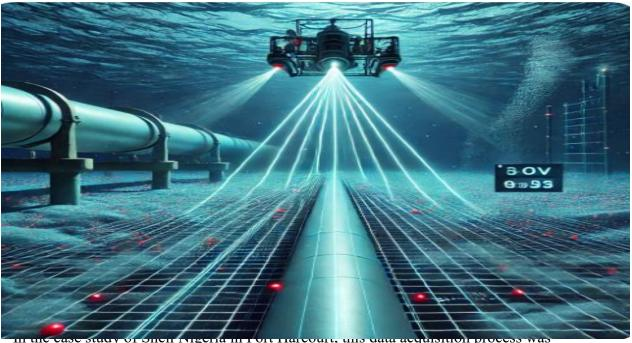
implemented along several key subsea pipelines transporting crude oil from offshore fields to onshore facilities. The challenging underwater environment in the Niger Delta, characterized by heavy sedimentation and high turbidity, provided an excellent opportunity to test the robustness of the LiDAR technology. The ROVs equipped with LiDAR sensors were able to penetrate the turbid water and scan the pipeline surface, collecting accurate and high-resolution data even in difficult conditions.
