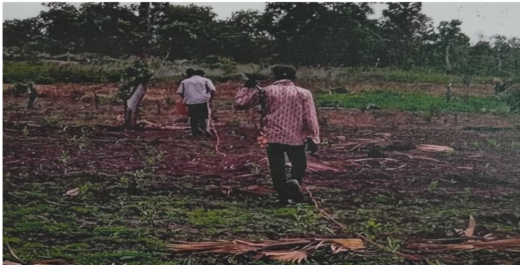
Plate 2: Laying of Surveying Cable in N-S Direction Across Inferred Structures in the Study Area
