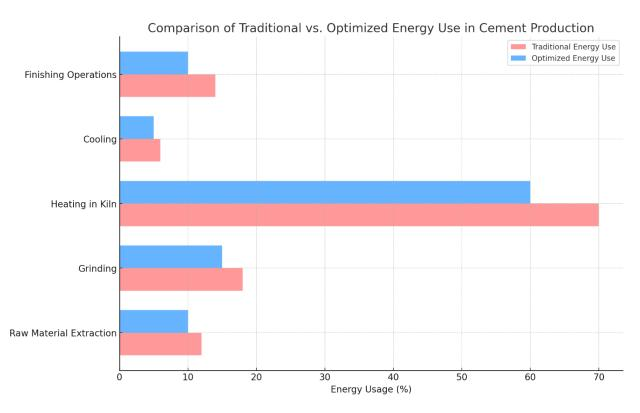
Here is a comparative diagram showing the differences in energy usage between traditional fixed schedules and optimized, AI-driven approaches in cement production:
