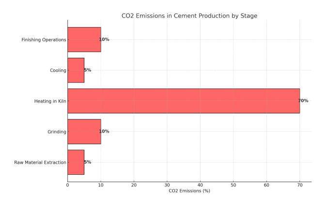
Here is a diagram that illustrates the contribution of different stages in cement production to overall CO2 emissions:
