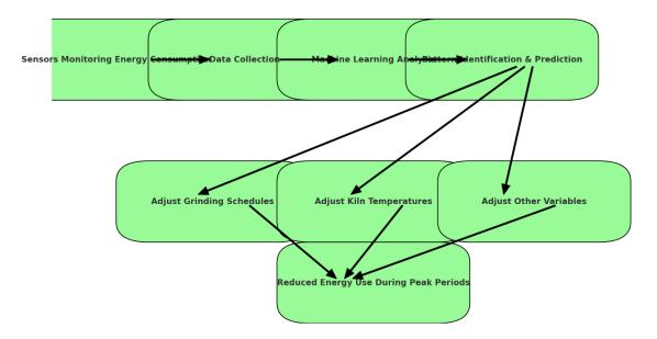
Here is a detailed diagram illustrating how a cement plant might use Machine Learning (ML) algorithms to analyze data from various sensors monitoring energy consumption across different stages of production:
