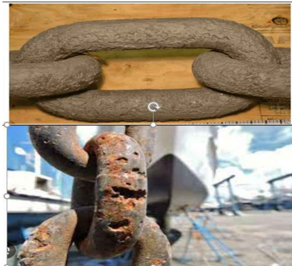
Figure (1): Pitting on mooring chains due to microbial induced corrosion (Source: Melchers, 2003)
