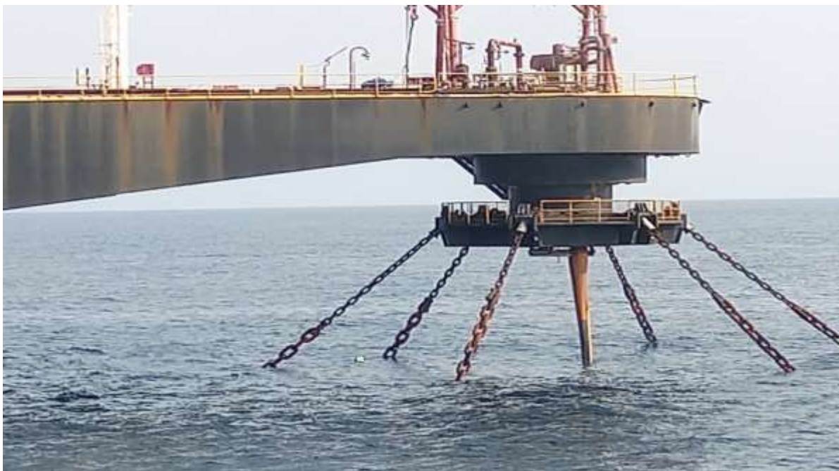
Figure (3): External turret mooring arrangement (Source: Maslin., 2013)
