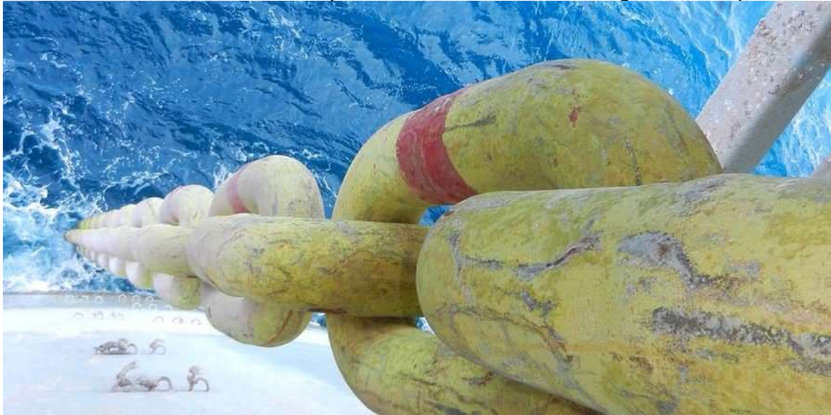
Figure (4): A Thermally sprayed aluminium coated mooring chains in operations (Source: Ma et al., 2019)
