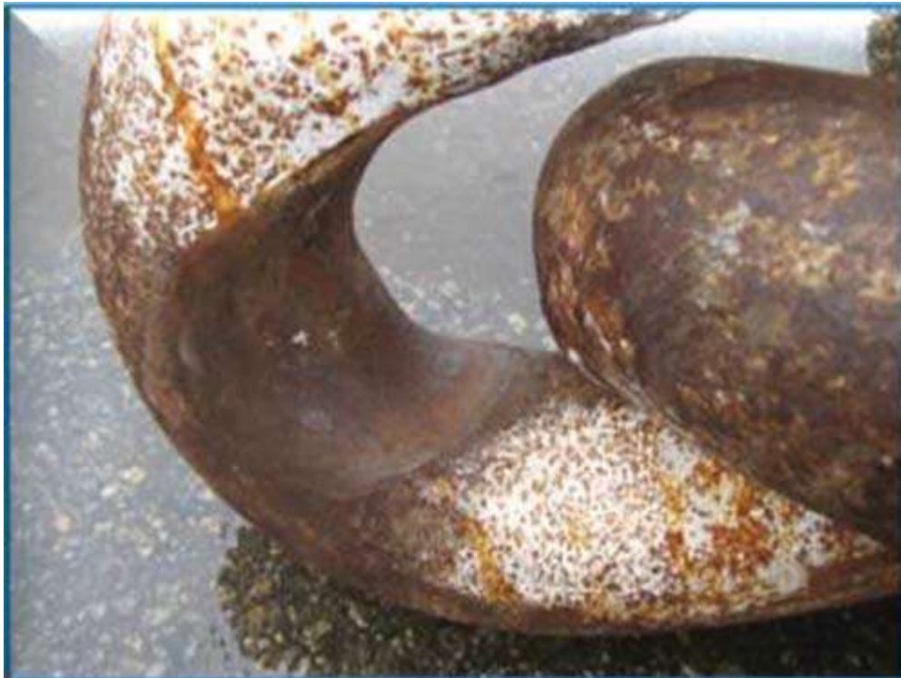
Figure (8): Wear and tear on chain link (Source: Birades and Verney, 2018; HSE, 2017)
