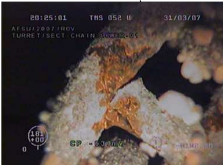
Figure (7): Partially loosened stud (Sharp and Ersdal, 2021)
