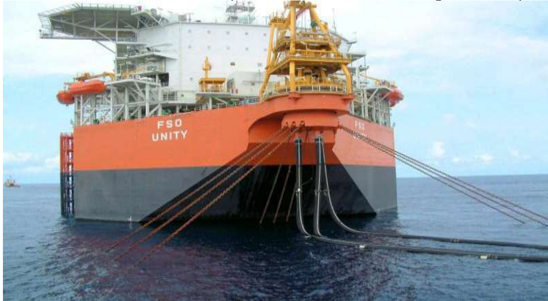
Figure (3): External turret mooring arrangement [18]
