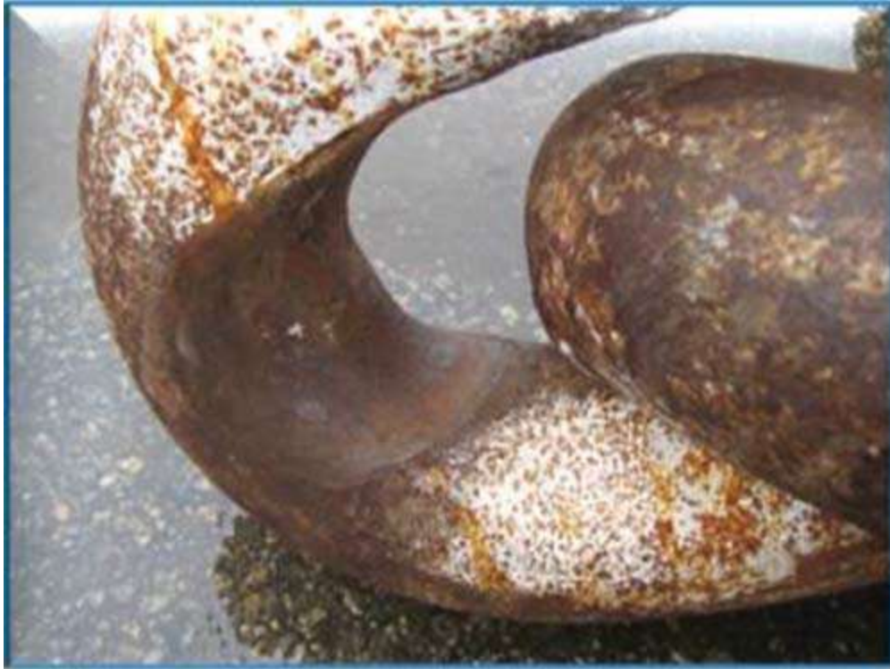
Plate (8): Wear and tear on chain link [91]
