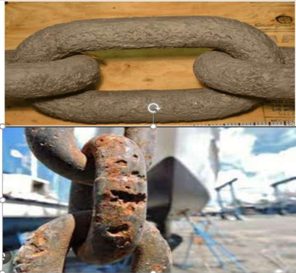
Figure (1): Pitting on mooring chains due to microbial induced corrosion [35]
