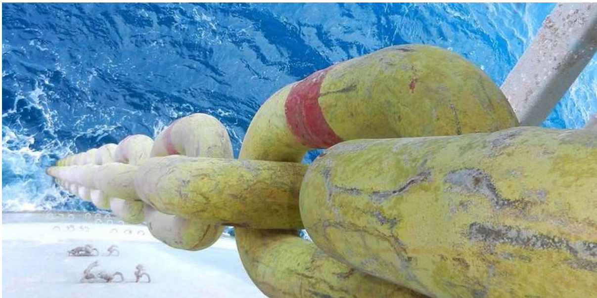
Figure (4): A Thermally sprayed aluminium coated mooring chains in operations [75]
