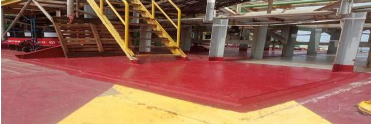
Figure (8): Composite repairs on FPSO main deck plate (Source: MOG, 2023)
