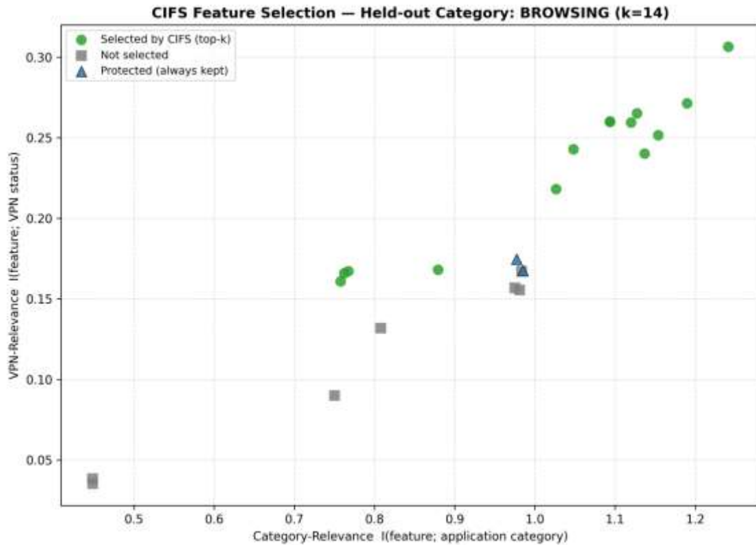
Figure 2. CIFS's dual-scoring and top-k selection illustrated for one representative held-out category (BROWSING, k=14 , matching Table 8). Each point is one feature, plotted by its category-relevance (x-axis) and VPN-relevance (y-axis); green points are the top-14 features by invariance score (VPN-relevance \div category-relevance) retained by CIFS, gray points are not selected, and blue triangles are the two throughput features always retained under Step 3.5 regardless of rank.
