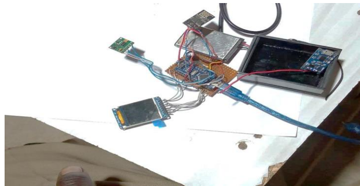
Plate 4: Vero board of developed AVSMDIoT
