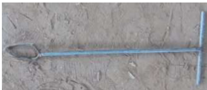
Figure 4 showing hand auger locally made for the collection of soil samples in the study area
