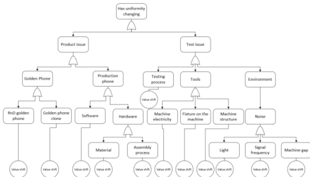
Figure 5. Fault Tree Analysis Causes of Data Uniformity Changes
