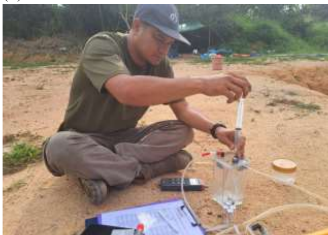
Figure 1: Field deployment of the recirculating gas sampling system (i), highlighting the battery-operated pumps (ii) and the manual extraction of headspace gas via syringe (iii).
