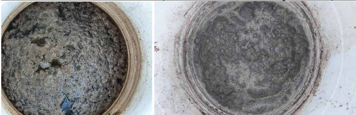
Figure 5: Foaming observed on slurry surface following reacidification processes
