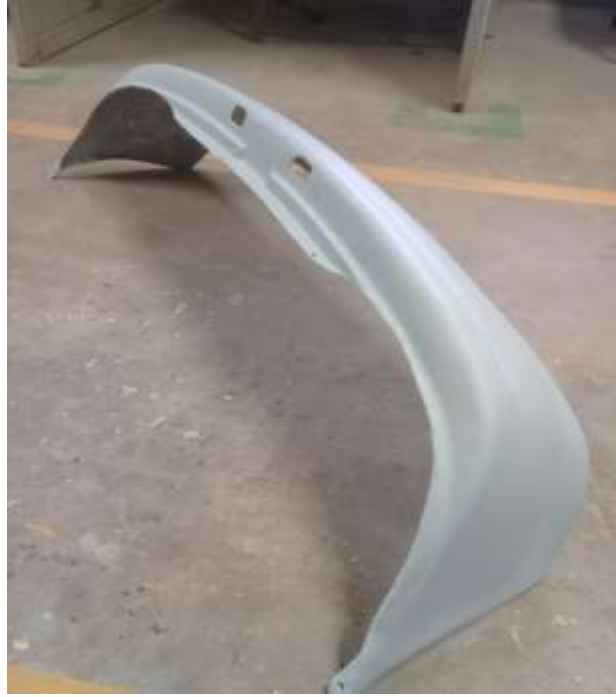
Plate X1: Finished composite bumper.
