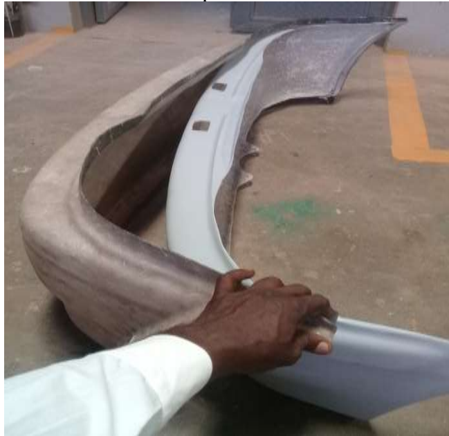
Plate X: Removal of cast bumper from the mould.
