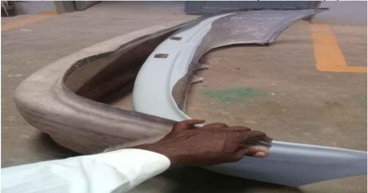
Plate IV: Removal of cast bumper from the mould.
