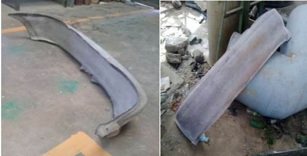
Plate VII: Fabricated bumper mould, (Inner and outer surface)
