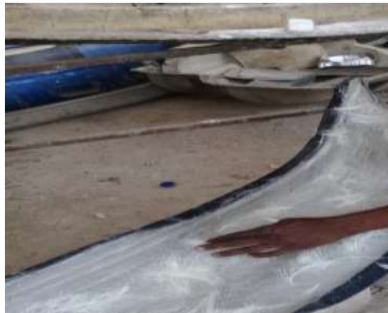
Plate VIII: Laying of fibre in the mould.
