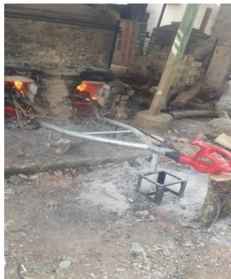
Fig. 14: The blower is being introduced
