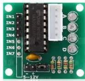
Fig 2.7: Uln2003 Engine Driver With Stepper Engine And Arduino (source: wikipedia.com)
