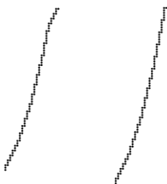
Figure19. Examples of SLRD accepted by the AFA of Fig. 17 with to = 5 . However they are not recognized by traditional methods without adaptivity.
